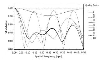
Figure 5. Ford's MTF results derived using the traditional edge technique. Diagram reproduced from reference [4].
