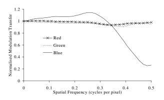
Figure 9. Calculated overall MTF for edge transitions in each of the red, green and blue colour channels compression using a quality factor of 90.
