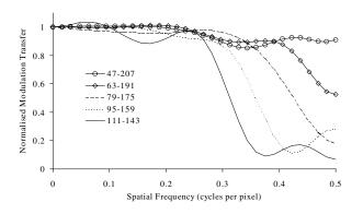
Figure 8. Responses using monochrome edges of varying magnitude compressed with a quality factor of 30.
