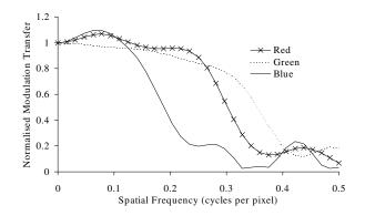
Figure 10. Calculated overall MTF for edge transitions in each of the red, green and blue colour channels compression using a quality factor of 30.
