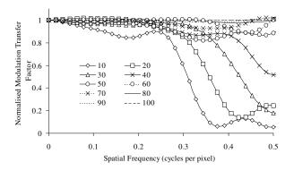
Figure 3. Measured MTF with respect to quality factor(10-100) for monochrome edges with a transition from 95 to 159 pixel values.
