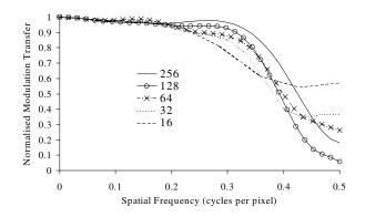
Figure 6. Variation in MTF with respect to the height of the region-of-interest selected (16-256 pixels) for an edge of transition 95 to 159 pixel values compressed using a quality factor of 30.
