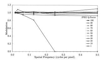
Figure 4. Ford's measurement of JPEG using a sine wave technique with respect to quality factor. Reproduced from reference [4].
