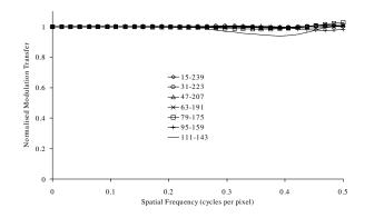
Figure 7. Responses using monochrome edges of varying magnitude compressed with a quality factor of 90.
